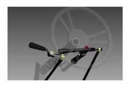
Unlike other Push/Right Angle controls, the Sure Grip Push/Right Angle's body does not pivot or move when the accelerator is applied. The pivot point for the Sure Grip control is on the left-hand side of the wheel, and only the handle pivots. A stationary main body has many benefits for the driver including:
