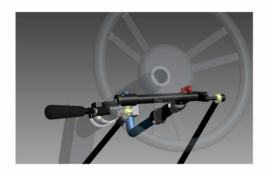
The Sure Grip Push/Pull hand control uses the same movement to apply the gas and brake as other Push/Pull controls; however, the pivot point for the Sure Grip control is on the left-hand side of the wheel, close to the handle. This allows for a shorter stroke and greater leverage. In addition to the pivot point, the handle's position is at a slight angle; an angle that makes a big difference to the driver. The benefits of Sure Grip's unique Push/Pull hand control design include:
